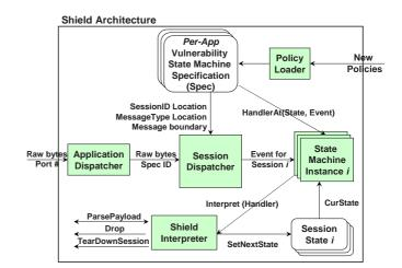
Figure 2: Shield Architecture
