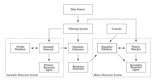
Figure 1: Hybrid immune based IDS model.
