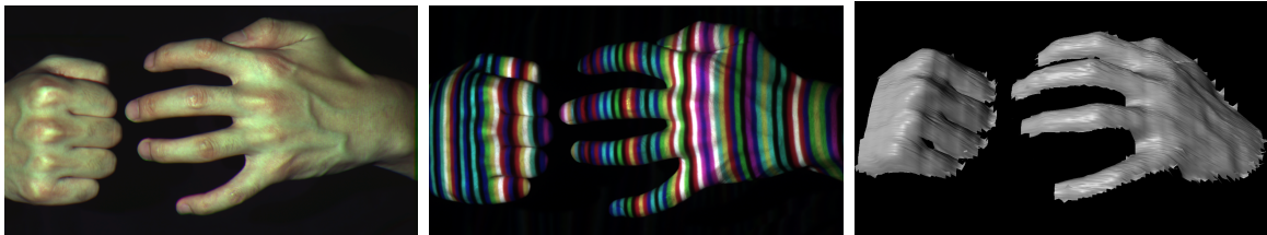
Figure 2.8: In this paper, we show how to reconstruct the shape of a scene, such as the two hands shown on the left, given a single photograph of the scene under color-striped illumination shown at center. A novel dynamic programming method leads to the geometric reconstruction on the right, shown as a shaded rendering from a new viewpoint.
