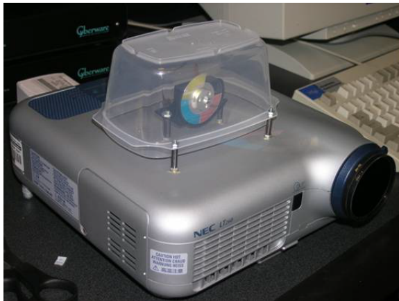
Figure 5.5: We build a near infrared projector by moving the projector color wheel outside and attaching a UV block filter and an IR pass filter in front of the projector lens.
