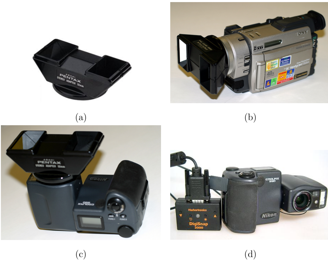
Figure 3.4: Single camera stereo with mirror adapter. (a) The Pentax stereo mirror adapter. (b) Sony TRV-900 camcorder mounted with the stereo adapter. (c) Nikon Coolpix-990 camera mounted with the stereo adapter. (d) Nikon Coolpix-990 with DigiSnap 2000 time lapse controller.
