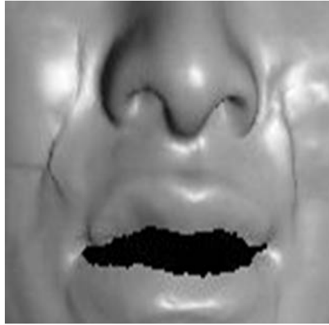
Figure 6.9: Bunching and folding artifacts in tracking results due to optical flow errors.
