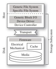
Figure 1: **The Storage Stack.** We present a schematic of the entire storage stack. At the top is the file system; beneath are the many layers of the storage subsystem. Gray shading implies software or firmware, whereas white (unshaded) is hardware.
