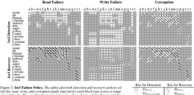
of workloads. The workloads are varied across the columns of the figure, and the different block types of the ixt3 file system are varied across the rows. The workloads are grouped in the same manner as in Figure 2.
