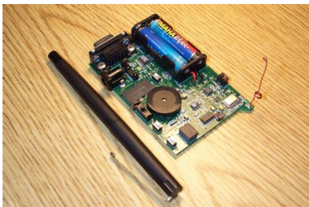
Figure 10: Prototype SpotON radio tag. These tags use radio signal attenuation to perform ad hoc lateration. Ad hoc clusters of tags cooperate to factor out measurement errors for all tag positions.
