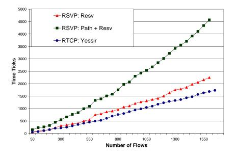
Figure 9: Protocol efficiency comparison between RSVP and YESSIR
