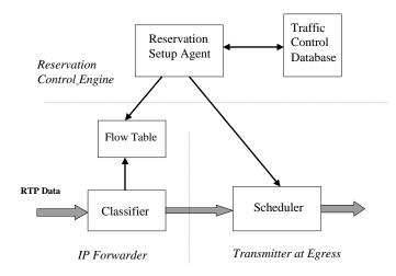
Figure 7: A router model for reservation support
