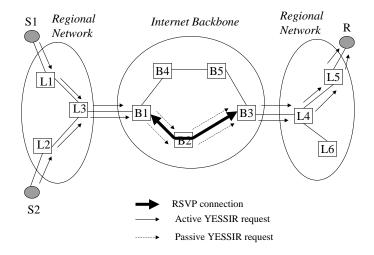
Figure 11: An example of solving the scaling problem with two levels of reservation
