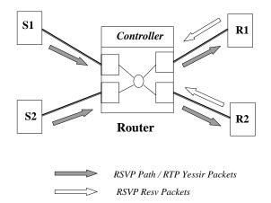
Figure 8: Set-up for studying RSVP and YESSIR processing costs
