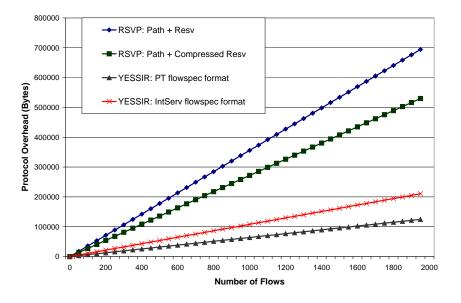
Figure 10: Protocol overhead comparison between RSVP and YESSIR
