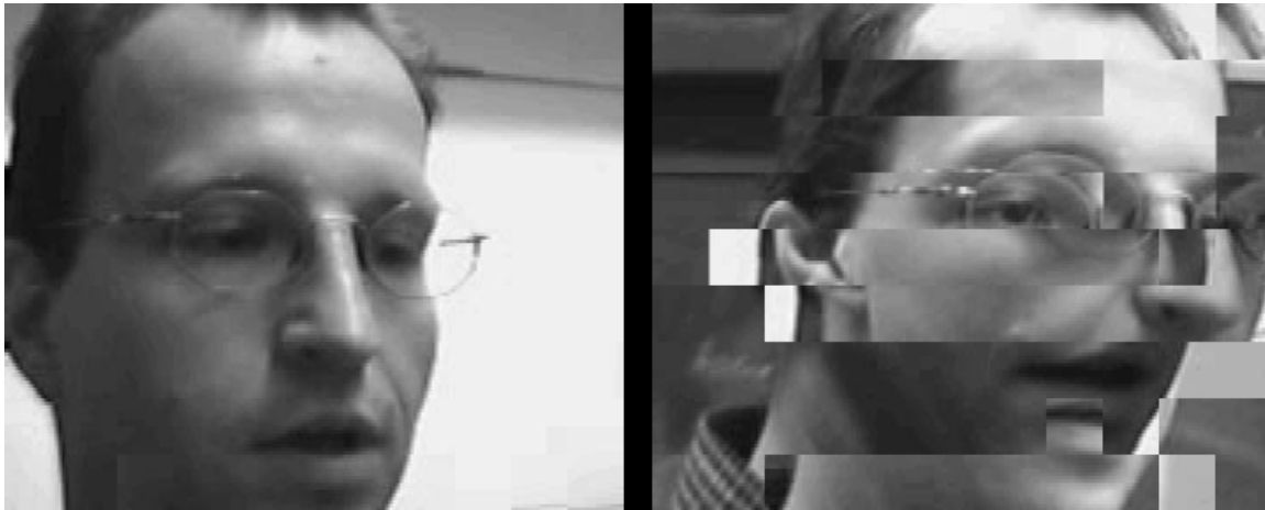
Figure 5. Transmission quality of an adaptive application with rate adaptation (lhs) and without rate adaptation (rhs).
