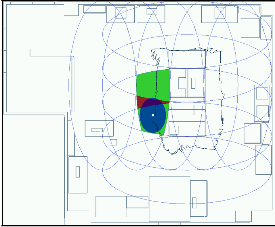
FIGURE 4. One of many tracked traversals of a rectangular path around the tables in the center of our lab: the “cell” fragment is dark grey, its lighter-grey superset fragment is the intersection, and the transparent grey ellipse with the white estimate dot at its centroid is the ellipse of confidence.
