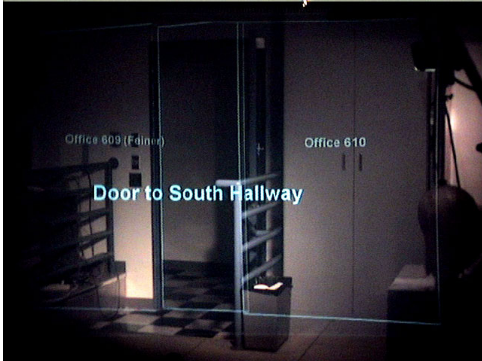
FIGURE 6. Augmented reality user interface in accurate tracking mode (imaged through optical see-through head-worn display). Labels and features (a wireframe lab model) are registered with the physical environment.
