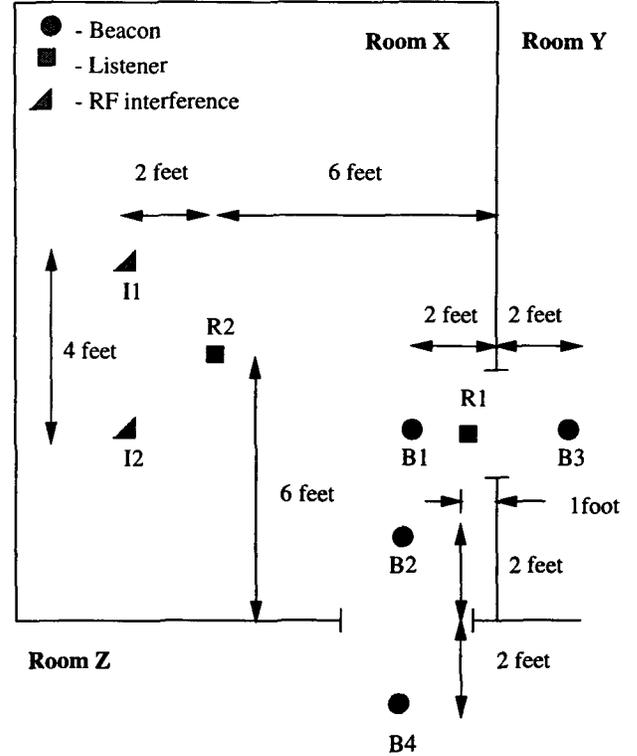
Figure 8: Setup for experiment 2, evaluating the robustness of Cricket in the presence of interfering beacons.
