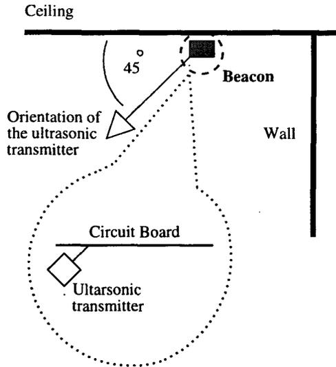
Figure 5: Correct alignment of a Cricket ultrasonic transmitter.
