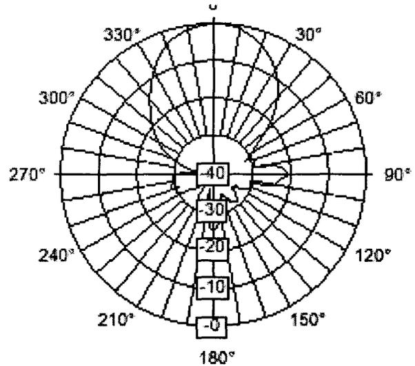
Figure 4: The radiation pattern of an ultrasonic transmitter.
