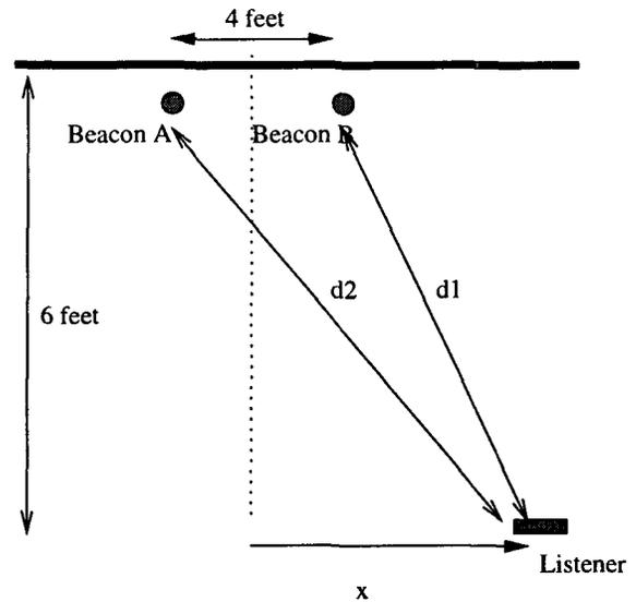
Figure 6: Setup for experiment 1, evaluating boundary performance.
