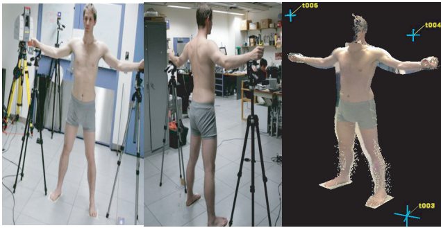
Figure 4: 3D model created by Cyclone. The slight movement during the scanning causes serious reconstruction problems
