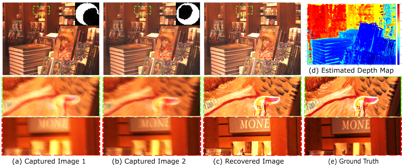
Figure 7. Inside a book store. (a-b) Captured Images using the coded aperture pair with close-ups of several regions. The focus is set at the middle of depth of field. (c) The recovered image with close-ups of the corresponding regions. (d) The estimated depth map without post-processing. (e) Close-ups of the regions in the ground truth image which was captured by using a small aperture f/16 and a long exposure time.
