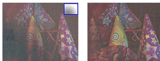
Figure 11: Application of the proposed post-processing algorithms to the dataset in [Veeraraghavan et al. 2007]. (Left) The original image. The inset shows the estimated vignetting field. (Right) The processed image. Image courtesy of Ashok Veeraraghavan.
