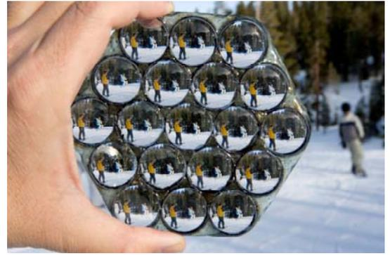
Figure 14: Picture of our hexagonal array of lenses and prisms.
