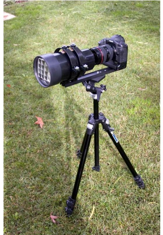
Figure 15: Working model of the camera in Figure 12, with 2 positive lenses and an array of 20 negative lenses.
