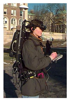
(a) The user wears a backpack and headworn display, and holds a handheld display and its stylus.
