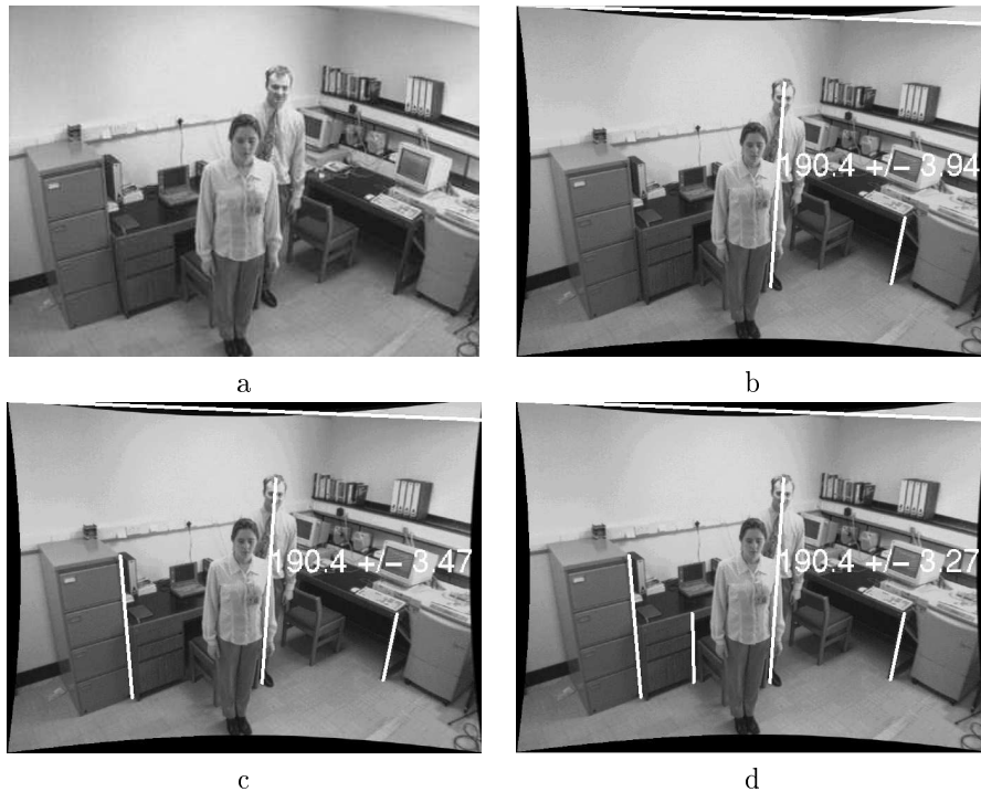
Fig. 16. Measuring heights and estimating their uncertainty: (a) Original image; (b) Image corrected for radial distortion and measurements superimposed. With only one supplied reference height the man's height has been measured to be Z = 190.4 \pm 3.94 cm, ( c.f. ground truth value 190cm). The uncertainty has been estimated by using (26) (the uncertainty bound is at \pm 3 std.dev.). (c) With two reference heights Z = 190.4 \pm 3.47 cm. (d) With three reference heights Z = 190.4 \pm 3.27 cm. Note that in the limit \Delta_P = 0 (error-free P matrix) the height uncertainty reduces to 2.16cm for all (b,c,d); the residual error, in this case, is due only to the error on the two end points.
