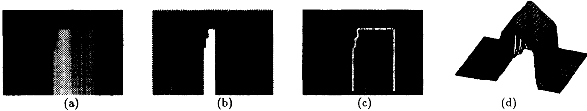
Figure 5: (a) Image of depth. (b) Image of slope. (c) Occluding contours and creases. (d) Wire frame of depth.
