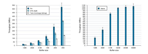
Figure 3.4: TCP socket throughput measured with *lmbench* for various buffer sizes. The numbers in the parentheses represent the additional bytes sent along with the real data, when using TaintExchange. We draw the mean and standard deviation. Note that the effect of Pin with the buffers drawn here is quite pronounced compared with the native execution of  $bw_tcp$ . Note though that the overhead diminishes as the size of the data read increases.
