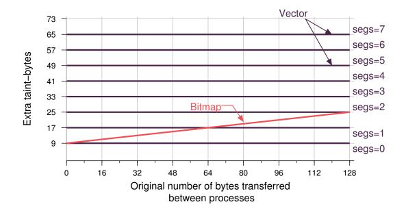
Figure 3.3: Space overhead of the different TaintExchange taint information transfer formats. For both formats, the fixed header size is 9 bytes. The overhead of the bitmap format is linear with the number of bytes transferred, while with the vector protocol it depends solely on the number of tainted data segments.
