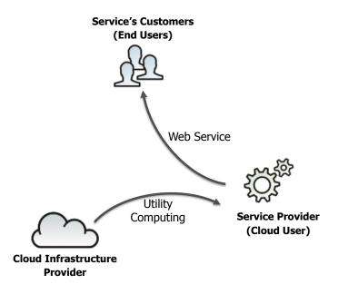
Figure 2.2: Cloud entities. The service provider uses the cloud infrastructure to deploy and host its service. End users access the service through its web interface.
