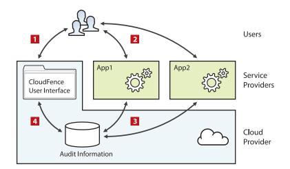
**Figure 4.1:** Main interactions between the different parties involved in CloudFence-enabled applications. Users register with the cloud provider (1), and then use the services offered by various service providers using the same set of credentials (2). Sensitive data is tagged and tracked transparently throughout the cloud infrastructure (3). Users can audit their data through a web interface exposed directly by the cloud provider (4).
