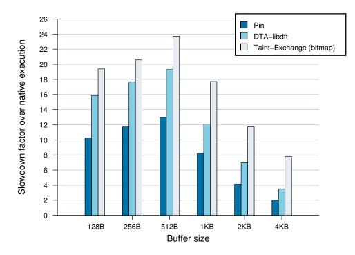
Figure 3.5: Slowdown factor in comparison with the native execution of bw\_tcp. Note that the native execution reaches a lower bound for buffers larger than 1KB (as seen in Figure 3.4). Therefore, the relative overhead for the three settings diminishes when reading these larger buffers.
