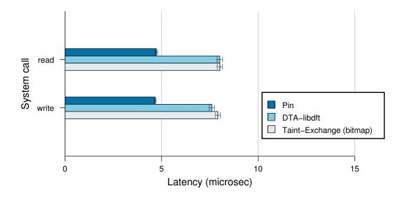
Figure 3.6: System call latency measured with *lmbench's* benchmark lat\_syscall. The buffer read and written is 1 byte. Note that the additional latency imposed by TaintExchange for write() system calls is due to the extra analysis that TaintExchange employs to determine whether the output stream is among the taint sinks.
