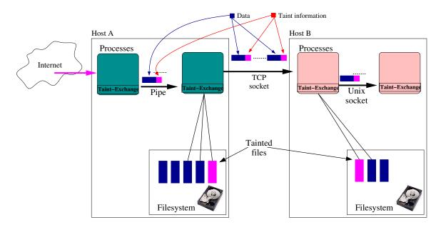
**Figure 3.1:** TaintExchange overview. Taint information can be exchanged using network sockets and pipes. Sockets and files can also be configured as taint sources.
