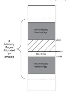
Figure 5. Example of pmalloc()-based memory allocation: the trailer and edge regions (above and below the write-protected pages) indicate "waste" memory. This is needed to ensure that mprotect() is applied on complete memory pages.
