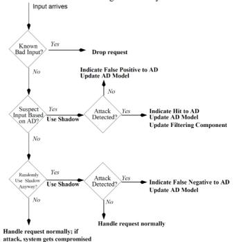
**Figure 3.** System workflow.
