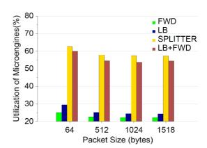
**Figure 11.** Utilization(%) of the IXP1200 Microengines, for forwarding-only (FWD), load-balancing-only (LB), both (LB+FWD), and full implementation (FULL), in stress-tests with 800 Mbit/s worst-case 64-byte-packet traffic.
