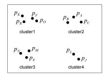
(b) Clusters of behavior profiles determined by the clustering algorithm. In this instance, four different clusters of behavior profiles have been identified by the central router among all hosts in the network.
