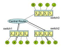
(a) Schematics of a network with multiple switches and hosts (circles). Each box within the switch represents a cluster-based AD sensor for each of the hosts in the subnet. The arrows indicate a traffic exchange from host A to host E.
