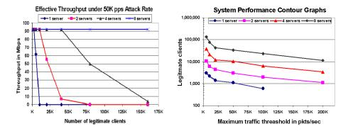
Fig. 5. (Left) Throughput of legitimate traffic under DDoS arrival rate of 50,000 packets per second. (Right) System performance contour graphs: we measured the maximum traffic threashold for different number of legitimate clients as we increase the amount of servers in a *gore* farm.
