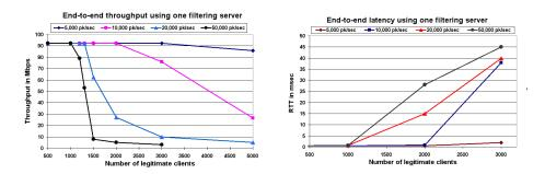
Fig. 4. (Left) Throughput of legitimate traffic with an average DDoS attack packet size of 1024 bytes  $\nu s$ . the number of legitimate clients. (Right) Round-trip time of traffic with an average DDoS attack packet size of 1024 bytes for different numbers of clients.
