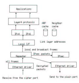
Fig. 3. the packet flow from the cipher port to the plain port
