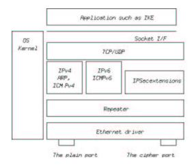
Fig. 1. the S/W module configuration
