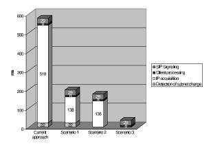
Fig. 8. L3 handoff time using SIP (average). Comparison between current approach and proposed approach (Scenarios 1, 2, 3)
