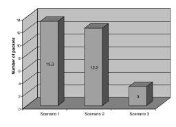
Fig. 10. Packet loss during L3 handoff (average)
