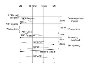
Fig. 9. Scenario 1: L3 handoff components and their delay
