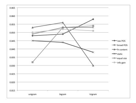
Figure 3.15: Logistic Regression accuracy using acoustic features and mixture model likelihoods from Uni-, Bi- and Trigram POS tags on BURNC.
