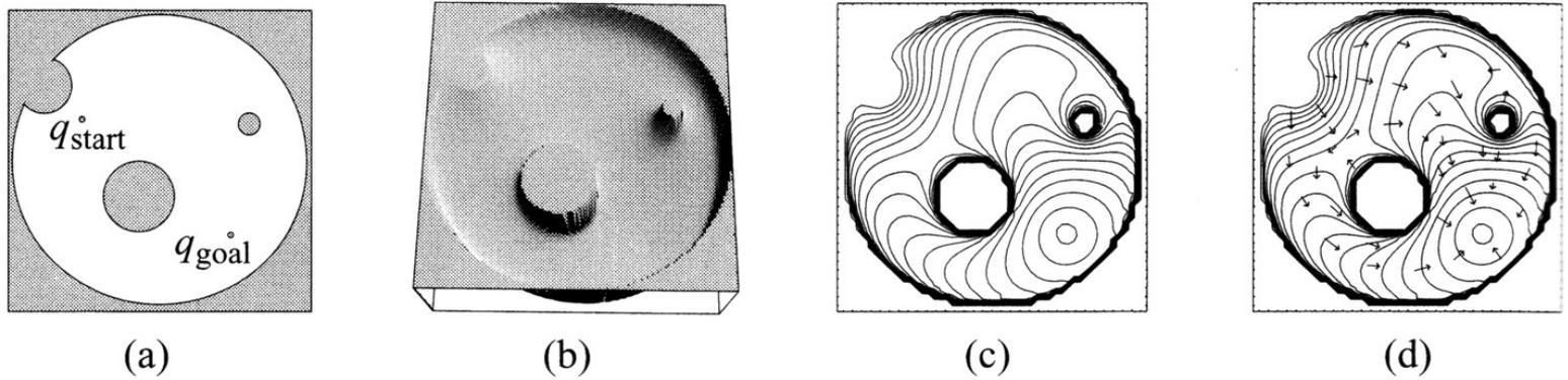
**Figure 4.3** (a) A configuration space with three circular obstacles bounded by a circle. (b) Potential function energy surface. (c) Contour plot for energy surface. (d) Gradient vectors for potential function.
