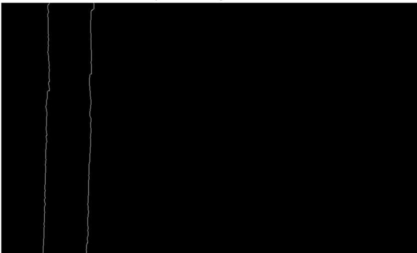
Canny edge detector applied to thresholded and masked yellow image
