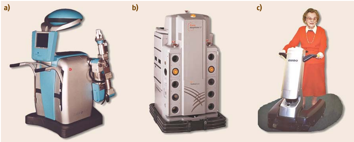
Fig. 53.6a–c Human assistance robots: (a) Care-O-bot, developed by the Fraunhofer Research Institute (Germany). (b) Helpmate by Transitions Research Inc., USA. (c) Pam-Aid (aka Guido), developed in the UK
