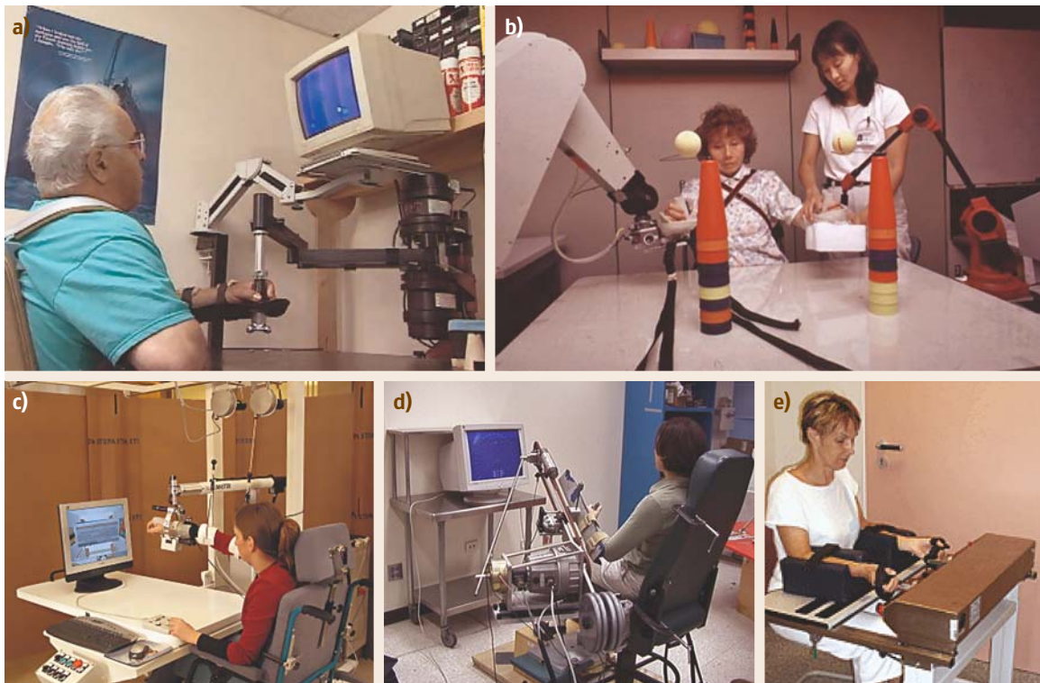
Fig. 53.1a–e Arm-therapy robotic systems that have undergone extensive clinical testing; (a) MIT-MANUS, developed by Hogan, Krebs, and colleagues at the Massachusetts Institute of Technology (USA); (b) MIME, developed at the Department of Veterans Affairs in Palo Alto in collaboration with Stanford University (USA); (c) GENTLE/s developed in the EU, (d) ARM-Guide, developed at the Rehabilitation Institute of Chicago and the University of California, Irvine (USA), and (e) Bi-Manu-Track, developed by Reha-Stim (Germany)
