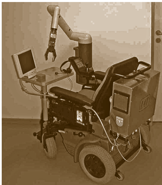
Fig. 53.4 Wheelchair manipulator robot MANUS developed at the Rehabilitation R&D Center, Hoensbroek, and marketed by Exact Dynamics (The Netherlands)
