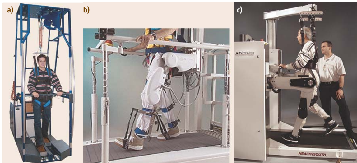
Fig. 53.2a–c Gait-training robotic systems currently in use in clinics; (a) the gait trainer GT-I, developed by Hesse's group and commercialized by Reha-Stim (Germany); (b) the Lokomat ® , developed by Colombo and colleagues and commercialized by Hocoma AG (Switzerland), and (c) AutoAmbulator ™ , developed by the HealthSouth Corporation (USA)
