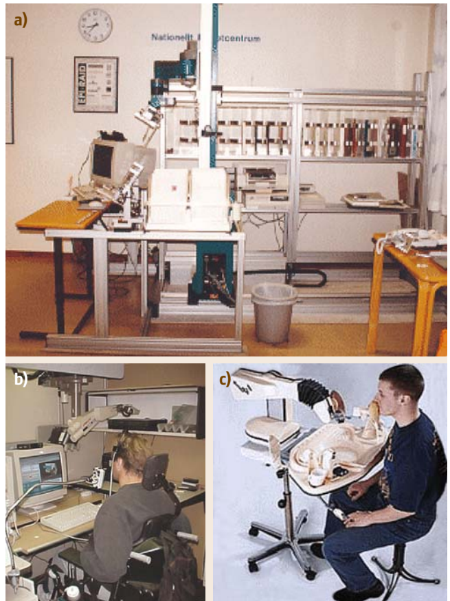
Fig. 53.3a–c Workstation-type robots: (a) AfMaster, developed by the French Muscular Dystrophy Association, (b) ProVAR, developed at the VA Palo Alto Rehabilitation R&D Center, and (c) Handy-1, developed by RehabRobotics, Ltd. (UK)
