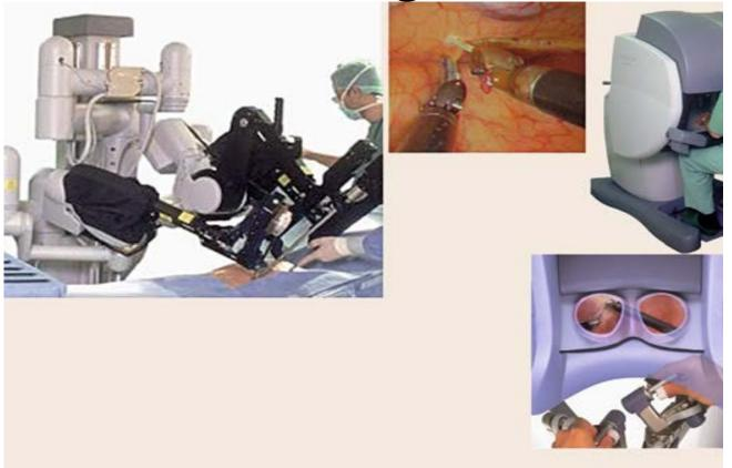
Robot arms to hold instrument Stereo display 6 DOF tool wrist Integrated master controller Standard laparoscopic paradigm –replaces human arms with robot arms
