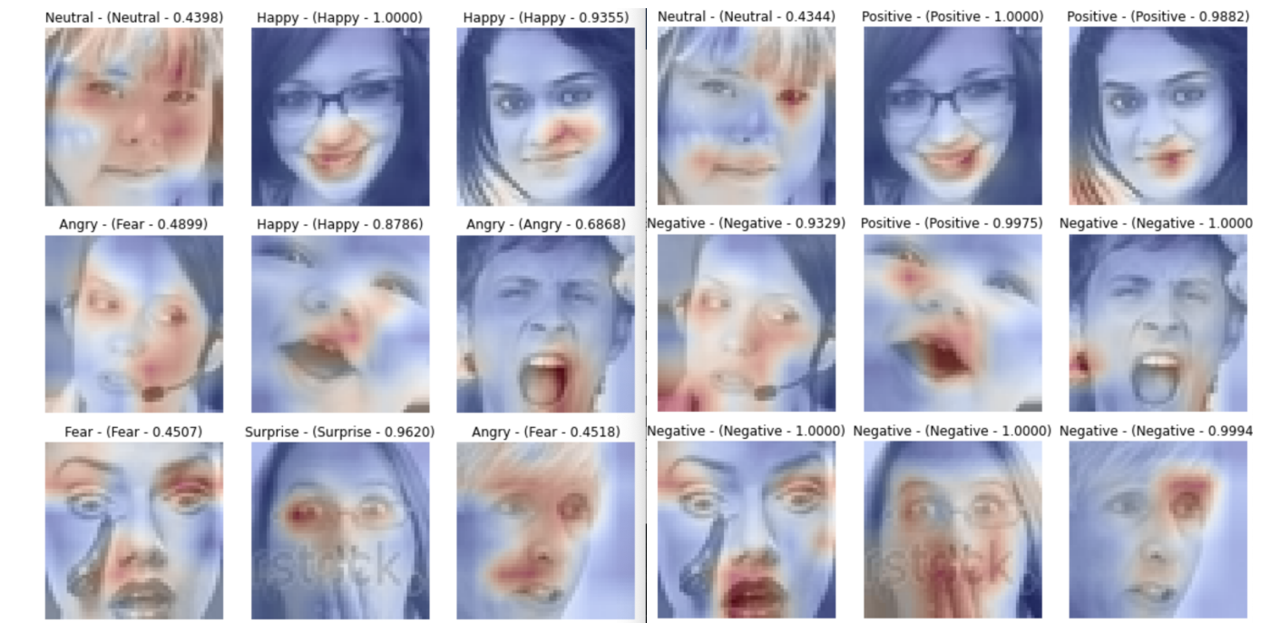
Figure 2. Contrast in attention heat maps across 9 random images: a CNN model trained on a 7-category dataset (left) vs. the same dataset categorized into 3 groups (right). Regions of high attention are shown in red.
