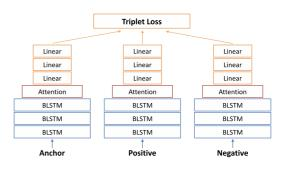
Figure 1: Siamese neural network with triplet loss.
