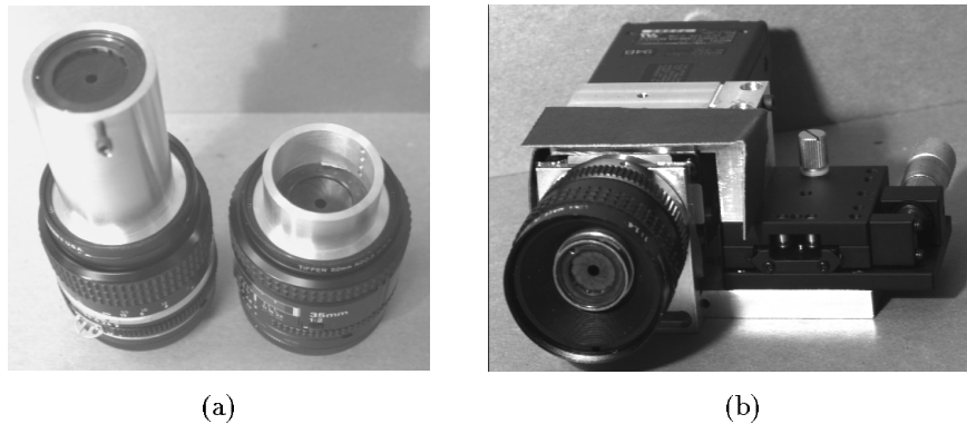
Fig. 4. Popular lenses converted into telecentric ones: (a) The Nikon Nikkor f=85\text{mm} SLR (left) and the Nikon AF Nikkor f=35\text{mm} SLR (right), and (b) The Fujinon CF12.5A f=25\text{mm} lens on a micrometer stage. In each case, the telecentric aperture resides in the aluminum casing appended to the front of the lens. The micrometer stage in (b) allows constant-magnification focus variation by displacing the image sensor from the lens.
