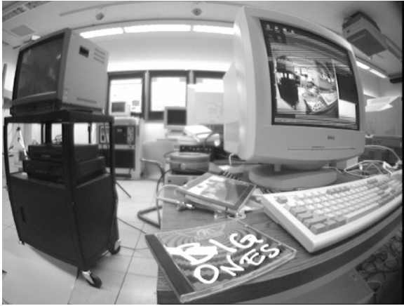
Fig. 1. Images captured with wide-angle cameras have severe distortions that alter the appearances of objects in the scene.
