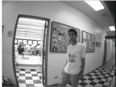
Figure 1: Images captured with wide-angle cameras have severe distortions that can alter the appearances of objects in the scene.
