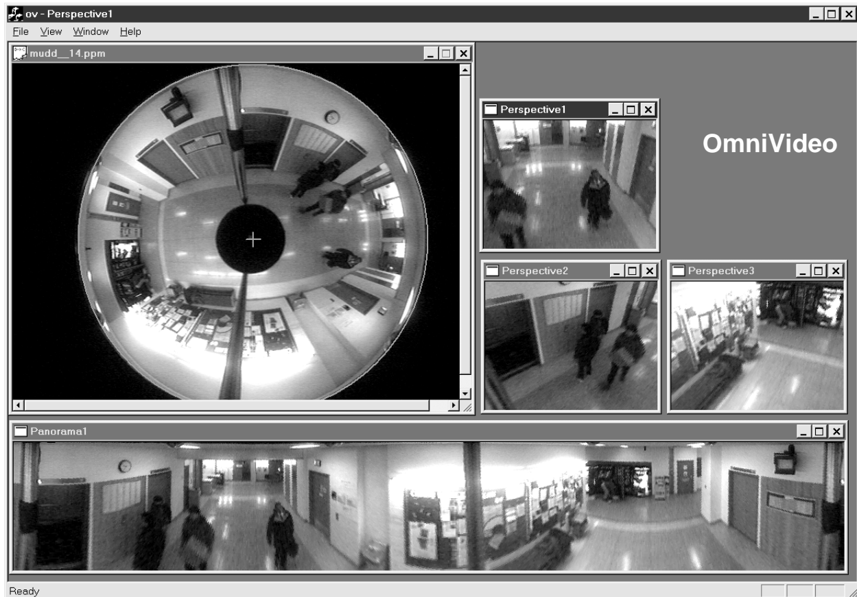
Figure 1: The OmniVideo system allows a user to generate multiple perspective and panoramic video streams from an incoming omnidirectional stream (top-left).
