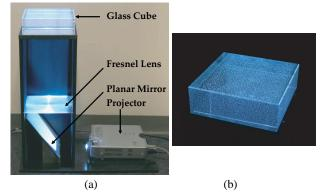
Figure 2: (a) An example implementation of the display system, including a light engine and an LID point cloud. (b) An example of a randomized LID cloud with  $48 \times 48 \times 25$  points in a  $200 \times 200 \times 70$ mm glass cube, uniformly lit by a projector.
