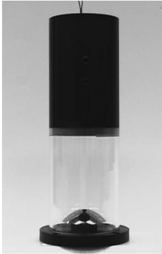
Figure 1: A compact omnidirectional camera that is 22 cm in height and 7 cm in width. This self-contained unit includes a video camera, telecentric optics and a curved mirror.
