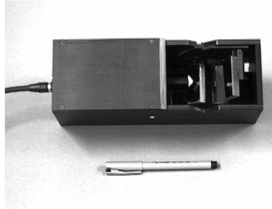
Figure 8: A compact catadioptric stereo camera that uses a single video camera and two planar mirrors. The positions and orientations of the planar mirrors can be adjusted by the user to alter the field of view based on the application. The planar motion constraint is used to robustly self-calibrate the device. A stereo algorithm has been developed that uses just a PC to produce 340x240 depth maps in real-time.
