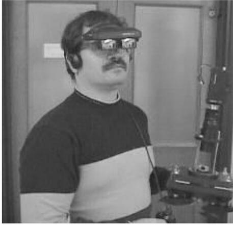
Figure 3: The remote reality system provides an immersive environment by combining an omnidirectional camera with a head-mounted display and head-tracker to produce perspective correct images as the user looks around.
