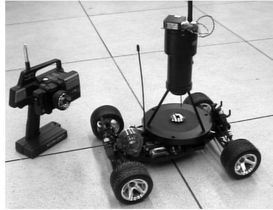
Figure 2: OmniRover: A remote-controlled car with an omnidirectional video camera, a microphone, a wireless video/audio transmitter, an FM receiver and speakers. A remote user can use the audio and video transmitted by the car to drive the vehicle, and communicate with people in a remote site.
