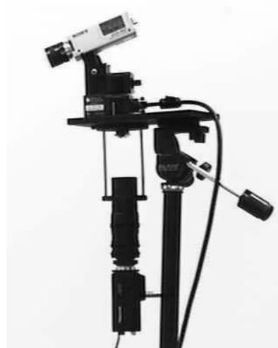
Figure 4: A combined wide-angle and narrow-angle imaging system. The omnidirectional camera provides a global view of the area of interest. Local regions are either automatically (via tracking) or manually (by user) selected from the global view and used as inputs to drive a pan/tilt/zoom system that produces high-resolution local views.
