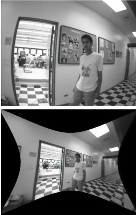
Figure 7: A non-metric algorithm has been developed for computing radial, decentering, and translational distortion parameters. A severely distorted image captured using a typical wide-angle lens (top). The (perspective) image after distortion correction (bottom). The distortion parameters can also be used to generate other projections such as panoramic or spherical.
