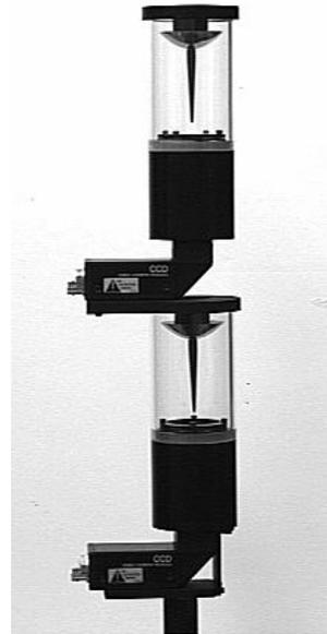
Figure 9: A panoramic stereo sensor. The sensor comprises of two identical omnidirectional sensing units. The optical axes of the two sensing units are aligned to ensure that the epipolar lines are radial in the captured images. An efficient stereo matching algorithm, implemented on a PC, computes panoramic depth maps in real time.
