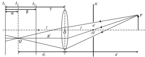
Figure 2: A constant-magnification imaging system for depth from defocus is achieved by simply placing an aperture at the front-focal plane of the optics.
