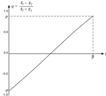
Figure 5: Relation between focus measures  $g_1$  and  $g_2$  and the defocus parameter  $\alpha$ .
