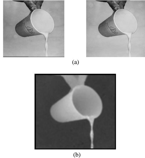
Figure 7: (a) Two images of a scene taken using different focus settings. (b) A depth map of the scene computed in 33 msec by the focus range sensor.
