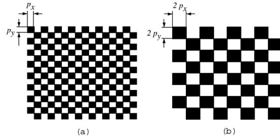
Figure 4: Optimal illumination filter patterns: (a)  $t_x = 2p_x, t_y = 2p_y, \varphi_x = 0, \varphi_y = 0$ ; and (b)  $t_x = 4p_x, t_y = 4p_y, \varphi_x = 1/8t_x, \varphi_y = 1/8t_y$ . Here,  $(t_x, t_y)$  is the illumination period,  $(p_x, p_y)$  is the pixel size, and  $(\varphi_x, \varphi_y)$  is the illumination phase shift with respect to the sensing grid.
