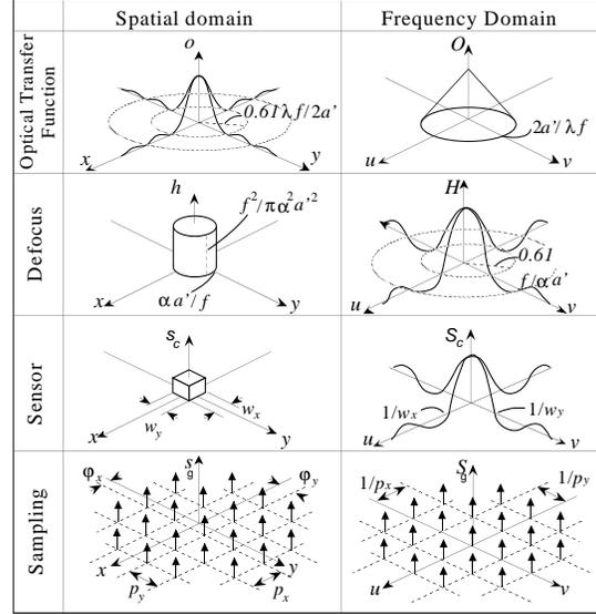
Figure 3: Spatial and frequency models for the optical and sensing elements of depth from defocus.
