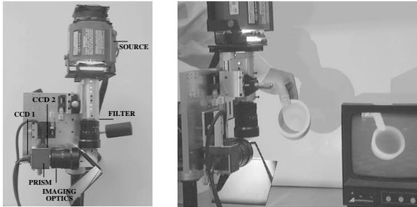
Figure 6: (a) The real-time focus range sensor and its key components. (b) The sensor can produce depth maps up to 512x480 in resolution at 30 Hz.
