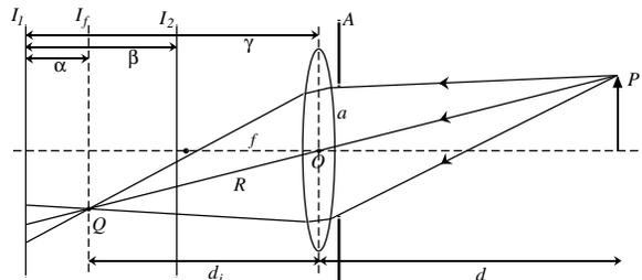
Figure 1: Image formation and depth from defocus.
