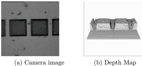
Figure 10: Image and depth map of rectangular structures on a smooth silicon substrate. The structures are approximately  $13\mu\text{m}$  tall.
