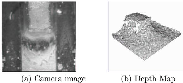
Figure 11: Image and depth map of a solder joint on a circuit board. The solder joint is approximately  $150\mu\text{m}$  high and  $100\mu\text{m}$  wide.
