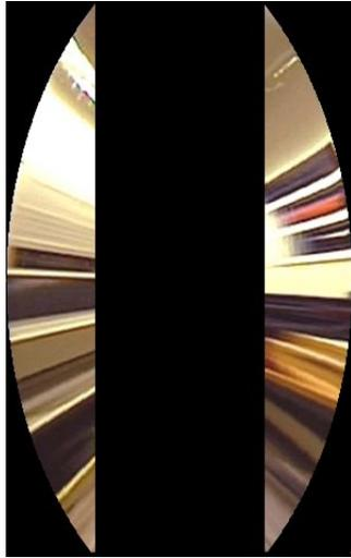
Figure 12: Two 90 degree sections of a cone are projected on to the larger dimension of the rectangular image. This results in a panoramic slice camera with a two-fold increase in slice resolution.
