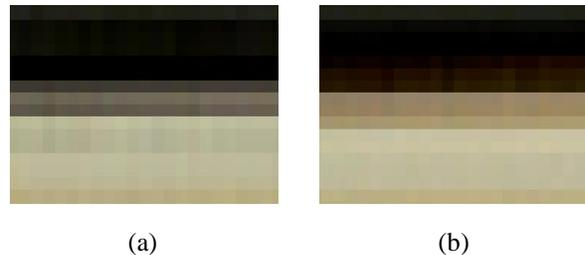
Figure 10: Magnified images of a step edge in the scene reconstructed using (a) an image disc of 1 pixel width and (b) an image disc of 4 pixels width. Note the effects of aliasing in (a).
