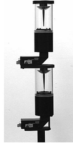
Figure 8: A compact panoramic stereo camera. In this design we used parabolas with a  $360^\circ \times 200^\circ$  field of view.
