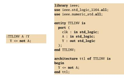
Figure 18: An inverter component defined in my HDL and the VHDL code I generate for it.
