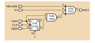
Figure 7: Circuit that generates the net
