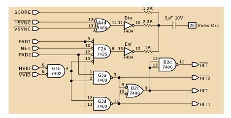
Figure 13: Video generation circuitry. F2b combines the signal from the two paddles, the net, and the ball. The score display is mixed with a 1.2K resistor, making it slightly dimmer.
