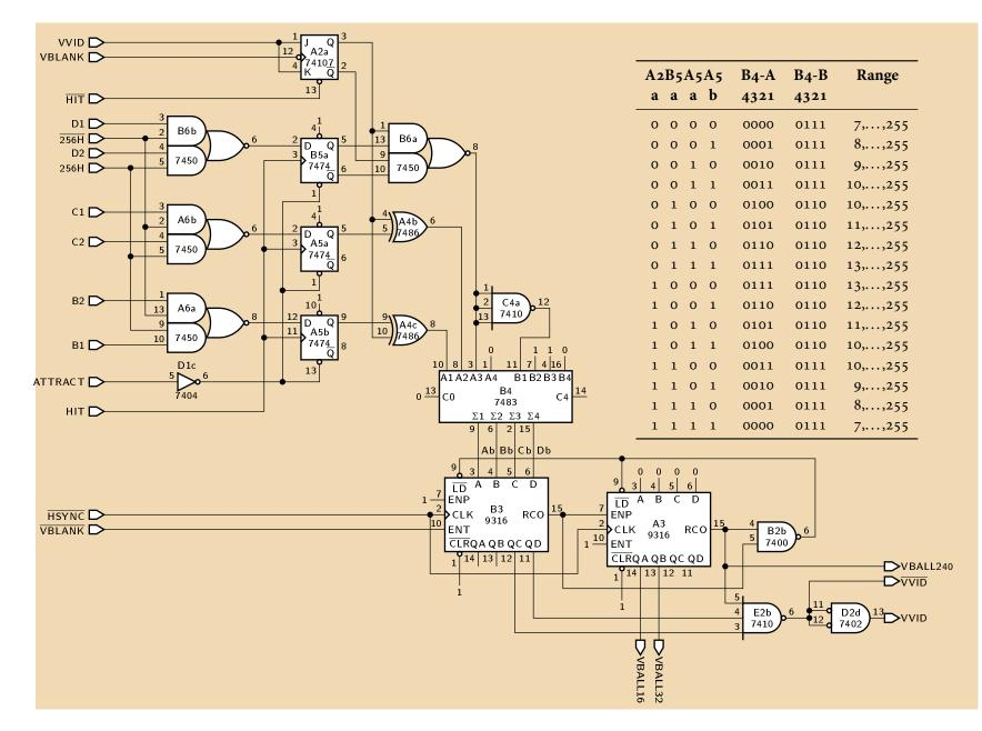
Figure 11: Ball vertical circuit. The output, VVID, is asserted when the ball is visible on the current line. Flip-flops B5a, A5b, and A5b remember the position at which the ball last hit a paddle; A2a toggles to rebound the ball off the top or bottom. Four-bit adder B4 translates the ball motion signals into a reset value for the eight-bit counter formed by A3 and B3, which determines the vertical position of the ball.
