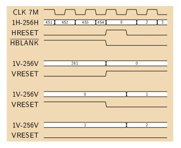
Figure 4: Behavior of the horizontal and vertical counters at the end of a horizontal line
