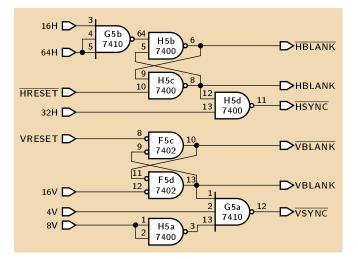
Figure 5: Horizontal and Vertical Blanking and Sync
