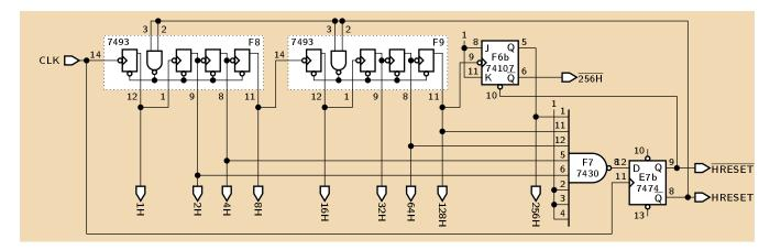
Figure 2: The horizontal counter: This counts 0, 1, ..., 454, generating a 15.734 kHz horizontal frequency.
