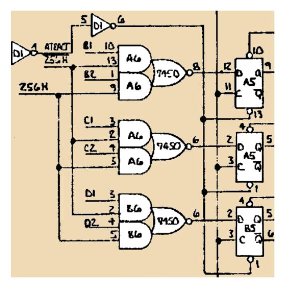
Figure 12: Part of *Pong*'s original schematic: the vertical ball counter. The intention of the top AND-OR-invert gate (A6) is clear: pass B1 under the same conditions as C1 and D1, but pins 1 and 10 are swapped: pins 1 and 13 are one group; 9 and 10 are the other.
