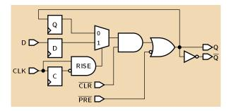
Figure 16: My circuit for emulating a 7474 positive-edge-triggered D flip-flop. The AND gate "RISE" detects a rising edge on the CLK input and either delivers the old Q output or the newly latched value of D.
