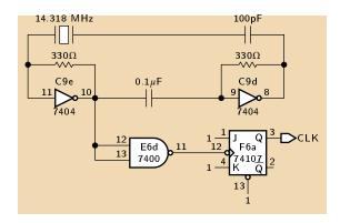
Figure 1: The main clock oscillator. This generates a 7.159 MHz square wave.
