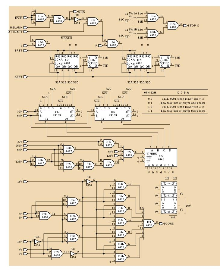
Figure 9: Score circuitry: the outputs of F5b and F5a pulse when a player has scored; C7, C8a, D7, and C8b maintain the score; the remainder displays the score as two two-digit seven-segment decimal numbers.
