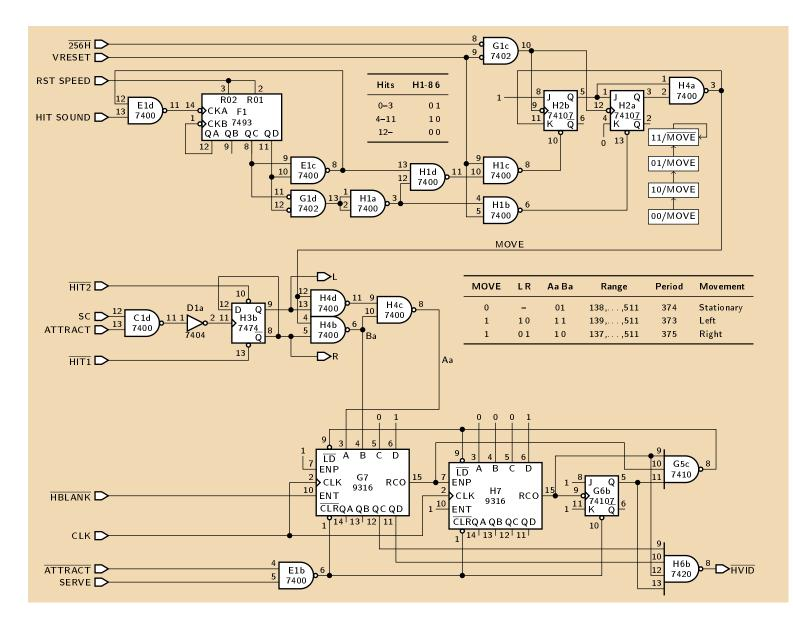
Figure 10: Ball horizontal circuit. The output,  $\overline{\text{HVID}}$ , is asserted when the ball is visible in the current column. Four-bit counter F1 counts hits and speeds up the ball in response. The duration of the MOVE signal controls how many pixels to move the ball left or right. Finally, the phase of the nine-bit counter formed by G7, H7, and G6b determines the horizontal position of the ball.
