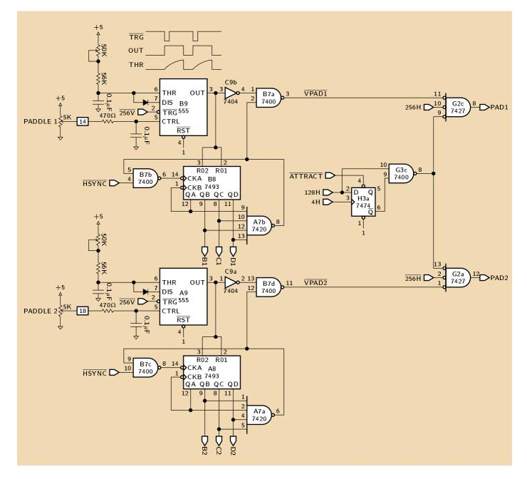
Figure 8: The paddle circuit. 555 timers A9 and B9 operate as one-shots triggered by  $\overline{256v}$  that select the top line of each player's paddle. Counters A8 and B8 and flip-flop H3a make each paddle 15 lines high and 4 pixels wide.
