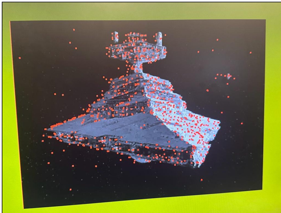
Fig. 10 - Final Output with the SIFT Annotated Key Points
