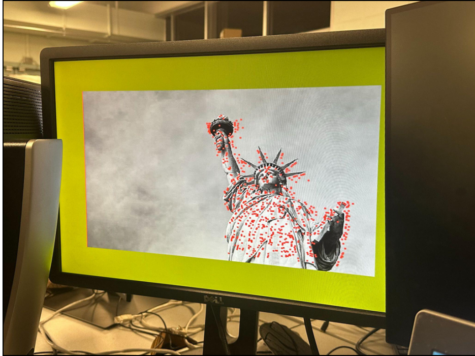
Fig. 09 - Final Output with the SIFT Annotated Key Points
