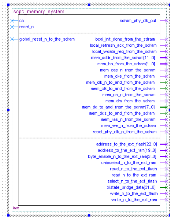
Figure 8–19. System Module with SDRAM and External Flash Memory
