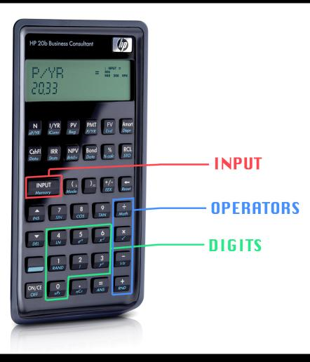
To carry out a simple operation, begin by typing your first operand into the keyboard. Then, press INPUT. The number you entered will appear on the LCD. Next, type out the second operand, and again press INPUT. Finally, press the operator you would like to use. The answer will then appear on the LCD.
