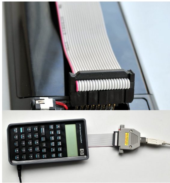
Figure 1: Connecting to the development ports on the back of the HP 20b calculator. Note that the jtag connector extends beyond the header.
