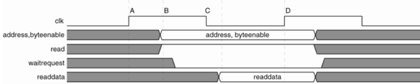
Figure 14: Fundamental Master Read Transfer with No Wait-States
