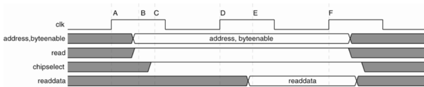
Figure 5: Slave Read Transfer with One Fixed Wait-State
