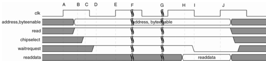
Figure 7: Slave Read Transfer with Variable Wait-States
