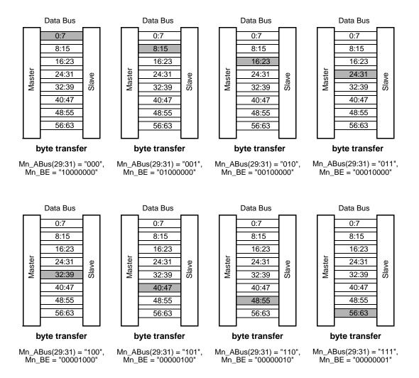
Figure 2-2: Byte lane usage for byte transfers
