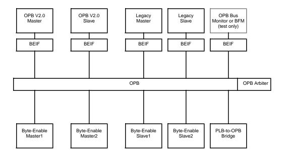
Figure 1-2: OPB Interconnect with Mixed Device Types
