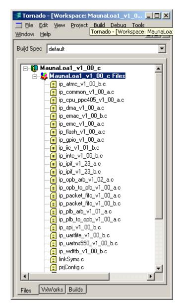
These files are prefixed with the name of the CSP. Figure 2 shows an example of the CSP build files.
