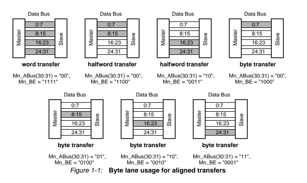
• All OPB slave devices that require a continuous address space (use of all byte lanes) will implement an attachment to the OPB bus that is as wide as the OPB data width, regardless of device width. This eliminates the need for left justification on the OPB bus and eliminates the need for masters to mirror write data.
