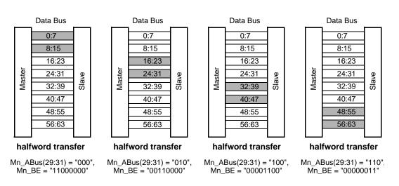
Figure 2-1: Byte lane usage for aligned doubleword, word, and halfword transfers
