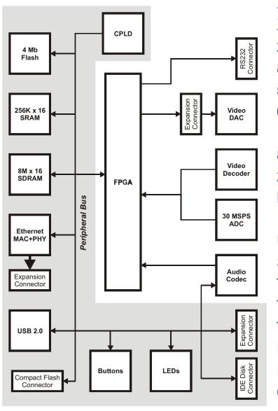
XC2S300E FPGA **XC9572 CPLD** 256K x 16 SRAM 8M x 16 SDRAM 512K x 8 Flash 6-channel NTSC video decoder 12-bit, 30 MSPS ADC 80 MHz, 30-bit video DAC 20-bit, 4-input, 1-output stereo codec Microphone/line-in/line-out jacks 10/100 Ethernet MAC+PHY USB 2.0 peripheral port Six pushbuttons, DIP switch Two LED digits, bargraph Three programmable oscillators Two expansion headers w/ 75 I/O pins Peripheral header w/ 18 I/O pins Parallel and Serial port **Compact Flash interface** IDE hard disk interface
