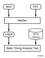
Figure 24-7: Static Timing Analysis Flow for FPGAs
