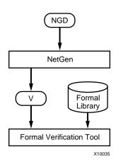
Figure 24-5: Post-Synthesis Flow for FPGAs
