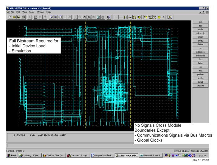
The following figure shows a routed design after the Final Assembly phase.
