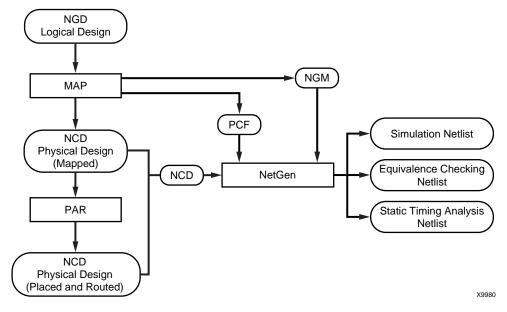
Figure 2-9: Back-Annotation Flow for FPGAs
