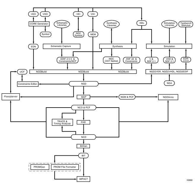
The following figure shows the Xilinx *software* flow chart for FPGA designs.
