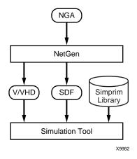
Figure 24-4: CPLD Timing Simulation
