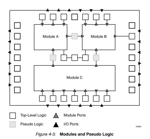
The following figure shows a detailed view of the pseudo logic shown in the preceding figure. In the figure, the output port for unexpanded Module A is connected to a pseudo load, and the input port for Module B is connected to a pseudo driver.
