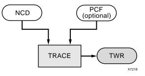
Figure 14-1: TRACE flow with primary input and output files
