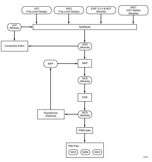
The following figure shows the flow through the Active Module Implementation phase:
