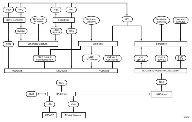
The following figure shows the Xilinx *software* flow chart for CPLD designs.
