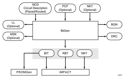
The following figure shows the BitGen input and output files:
