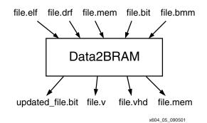
Figure 26-1: Data2MEM Input and Output Files
