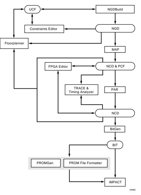
The following figure shows the design implementation process for FPGA designs:
