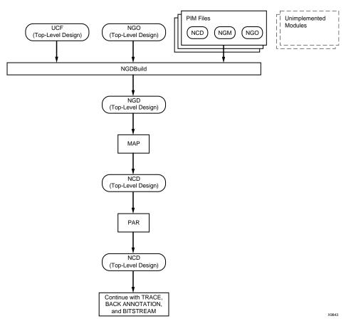
Figure 4-8: Final Assembly Phase for Partial Design Assembly Flow
