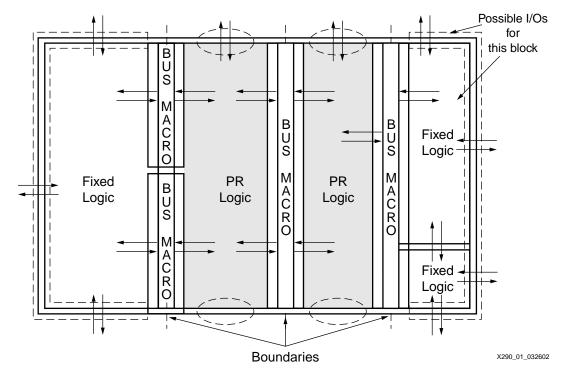
A layout of a design with two modules that are reconfigurable (shaded) is shown in the following figure.
