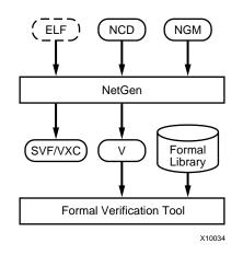
Figure 24-6: Post-Implementation Flow for FPGAs
