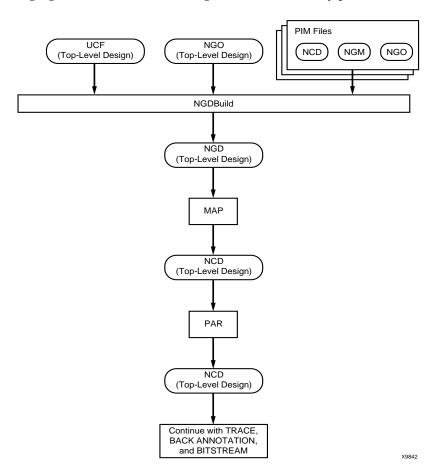
The following figure shows the flow through the Final Assembly phase.
