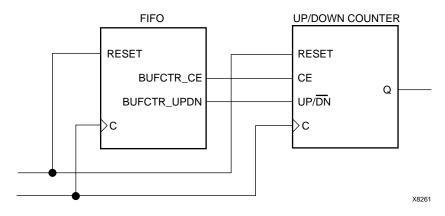
Figure 14-3: Clock Passing Through Multiple Buffers
