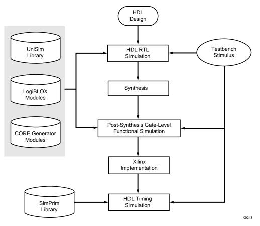
The following figure shows when you can perform functional and timing simulation:
