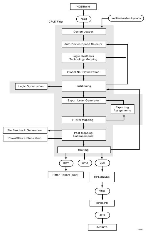
The following figure shows the design implementation process for CPLD designs:
