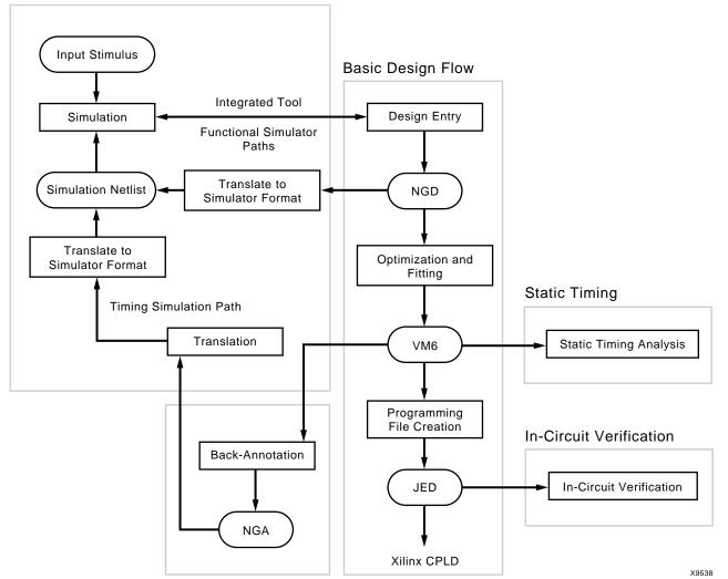
The following figure shows the verification methods of the design flow for CPLDs.
