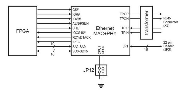
Packets will be constructed and transmitted according to the Ethernet Protocol. We will be initializing and interfacing with the controller through the control registers outlined in the datasheet of the AX88796
