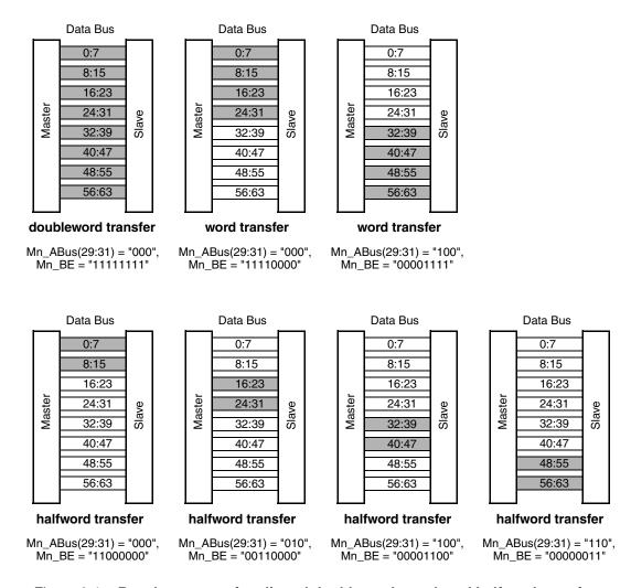
Figure 2-1: Byte lane usage for aligned doubleword, word, and halfword transfers
