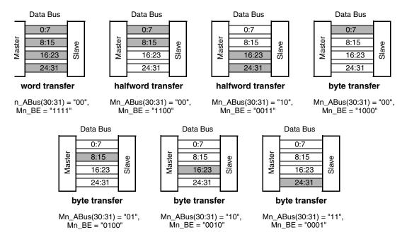
Figure 1-1: Byte lane usage for aligned transfers
