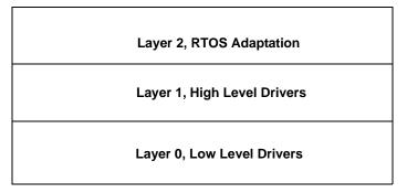
Figure 10-1: Layered Architecture
