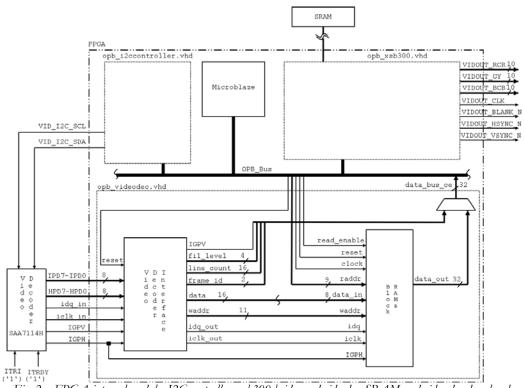
Fig. 2 – FPGA internal modules I2C controller, xsb300 bridge and videodec; SRAM and video decoder also shown.
