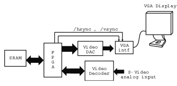
Fig. 1 - Obtrack block diagam.
