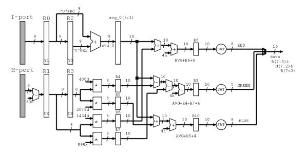
Fig.9 – YUV to RGB color space conversion implemented in the video decoder interface module.
