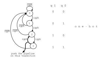
Fig.10 – Control state machine for the YUV to RGB pipeline shown in Figure 9.
